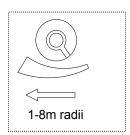
Reach is the term used to describe the radii of the more or less circular detection zone produced on the ground after mounting the sensor light at a height of 2.5m, turn the reach control fully anticlockwise to select minimum reach (approx.1 m radii), and fully clockwise to select maximum reach (approx. 8m radii).
